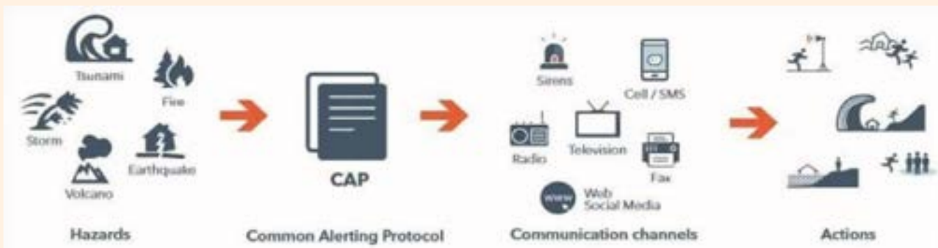
Figure 2-1: The Common Alerting Protocol.
