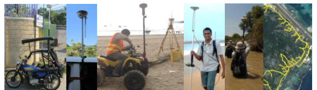
Figure 4. RTK GPS survey along road network, shoreline, and mangrove
