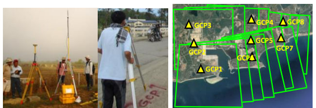
Figure 3. Baseline and PPK GPS survey for GCPs used in photogrammetry
