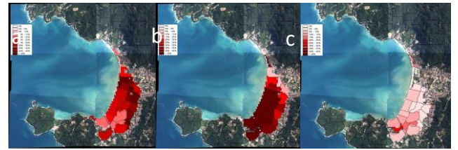
Figure 11. Probability of damage to one-story RC building for (a) secondary member, (b) primary member, (c) collapse
