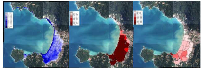
Figure 10. (a) Inundation height, probability of building damage to RC > 1 floor for (b) secondary member, (c) primary member
